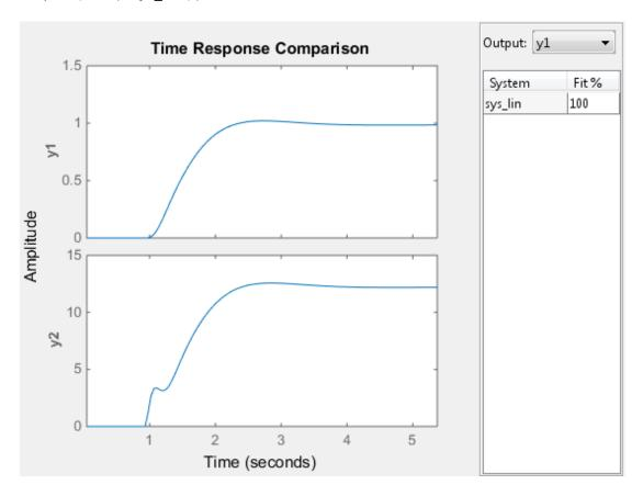
Because the data was obtained by simulating the linearized model, there is a 100% match between the data and model linearization response.
