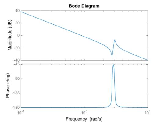
The cell array {0.1,10} specifies the minimum and maximum frequency values in the Bode plot. When you provide frequency bounds in this way, the software selects intermediate points for frequency response data.
