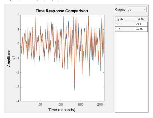
The regularized model m2 produces a better fit than the unregularized model m1.
