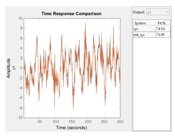
sys refines the estimated model and provides a 74.54% fit to the estimation data (see init sys.Report.Fit.FitPercent).
