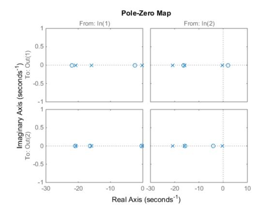
By default, the plot displays the poles and zeros of each I/O pair on its own axis. Use the plot handle to view all I/Os on a single axis.
