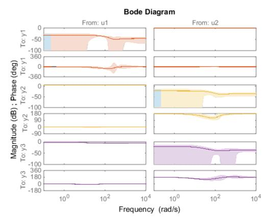
The confidence bounds for M2 overlap with those of m1, m2 and m3 models on their respective plot axes.
