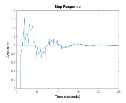
The system step response displayed is chaotic. The step response of systems with internal delays may exhibit odd behavior, such as recurring jumps. Such behavior is a feature of the system and not software anomalies.
