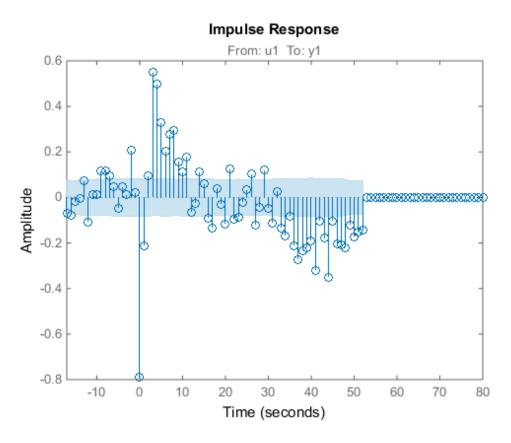
The large response value at t=0 (zero lag) suggests that the data comes from a process containing feedthrough. That is, the input affects the output instantaneously. There could also be a direct feedback effect (proportional control without some delay that u(t) is determined partly by y(t)).
