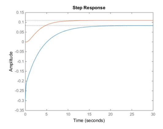
Each step response settles at a different steady-state value. Use the plot handle to normalize the plotted response.
