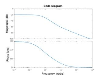
bode (sys1,...,sysN) plots the frequency response of multiple dynamic systems in a single figure. All systems must have the same number of inputs and outputs.
