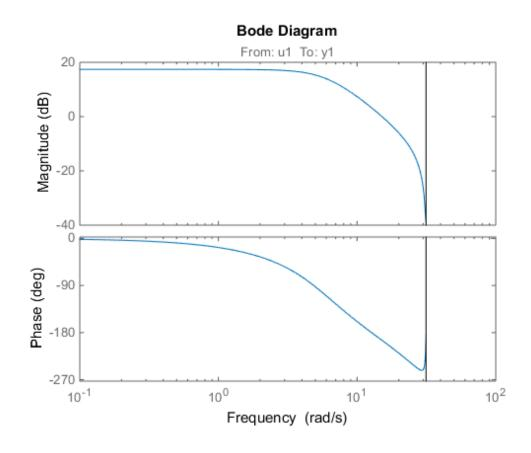
z1 is an iddata object that contains time domain system response data. SyS is an idpoly model containing the identified polynomial model. h is the plot handle for the bode response plot of SyS.
