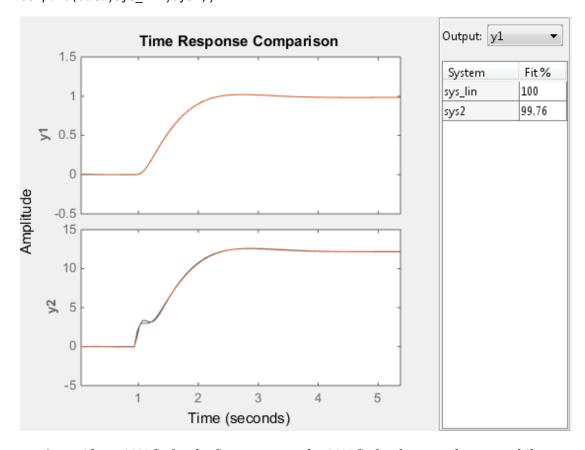
sys2 provides a 99% fit for the first output and a 98% fit for the second output while using 4 less states than sys\_lin.
