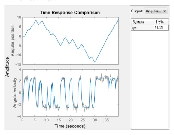
${\tt sys}$  provides a 98.35% fit for the angular position and an 84.42% fit for the angular velocity.
