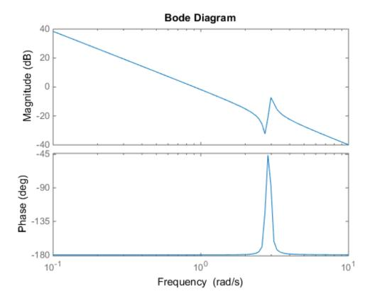
logspace defines a logarithmically spaced frequency vector in the range of 0.1-10 rad/s.
