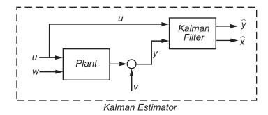
The block implements the steady-state Kalman filter when the system matrices (A(t), B(t), C(t), D(t), G(t), H(t)) and noise covariance matrices (Q(t), R(t), N(t)) are constant (specified in the Block Parameters dialog box). The steady-state Kalman filter uses a constant matrix P that minimizes the steady-state estimation error covariance and solves the associated continuous-time algebraic Riccati equation:
