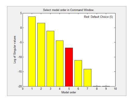
States with relatively small Hankel singular values can be safely discarded. The plot suggests using a fifth-order model.
