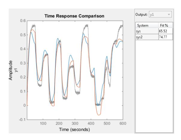
where sys2 refines the parameters of sys to improve the fit to data.
